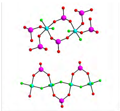
Figure. Ball-and-stick representation of gallium fluoride iodate unit of Li-complex (top) and Rb, Cs-complexes (bottom) (cyan, Ga; pink, I; green, F; and red, O).
