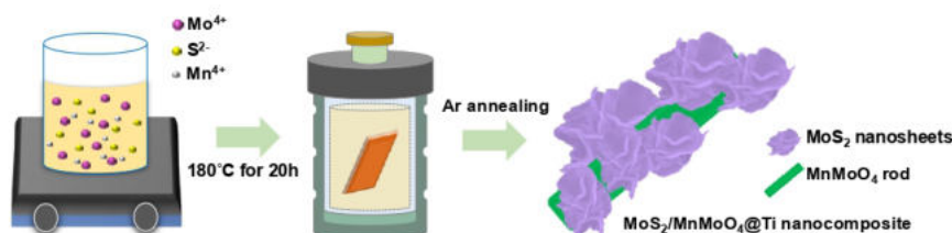
Scheme 1. Schematic illustration of the synthesis process for the MoS 2 /MnMoO 4 @Ti nanocomposite.
